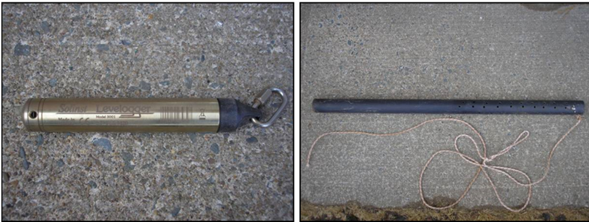
Figure 13 Solinst Levelogger (Model 3001) on the left and still well on the right. Photographs taken by N. Neatt, 2007.
